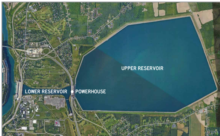
The Lewiston Pumped Storage Project is comprised of a massive upper reservoir, covering three square miles, and a pump station/power plant. It is part of the bigger Niagara Power Project. Base map: Google Earth image
